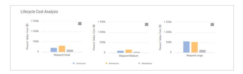
Despite being able to capture eight times more runoff than the medium wetpond, the large wetpond does not provide water quality benefits that justify the cost of such a large project. The large wetpond is simply oversized for the project area.
